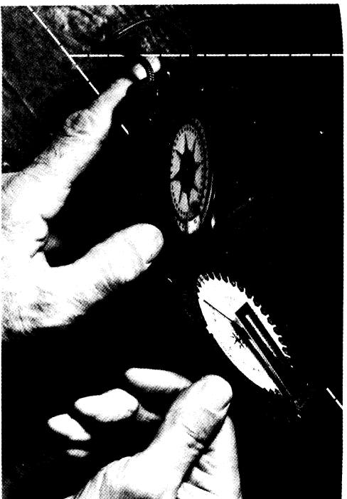
Fig. 5.13 Measuring lineation on a steep surface with a hinged-lid compass (see text).
