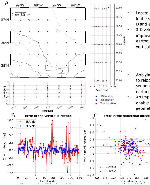
Locate 140 synthetic earthquakes in the study area based on the 1-D and 3-D velocity model. 3-D velocity model enable us to improve the accuracy of the earthquake location, especial in vertical direction.
